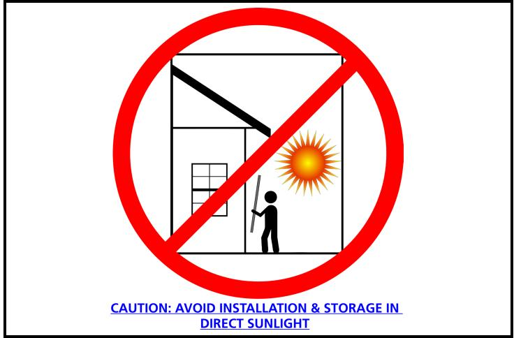
As with most building products certain precautions should be taken to minimize potential problems with thermal expansion or contraction during installation and/ or storage caused by direct exposure to sunlight, particularly during hot summer months.
