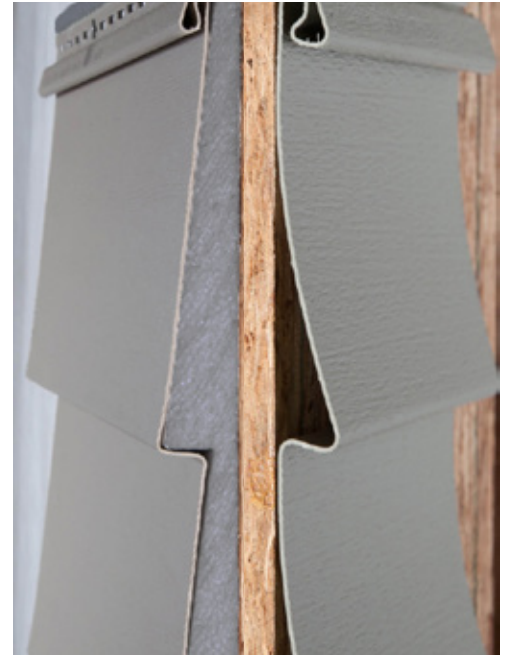
Siding supported with contoured insulation (left) maintains straight lines like real wood, while unsupported vinyl siding (right) can appear curved.
