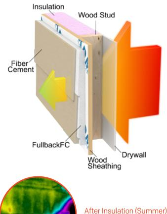
Thermal imaging reveals that the wall is a significantly cooler green with the addition of insulation to the exterior.
