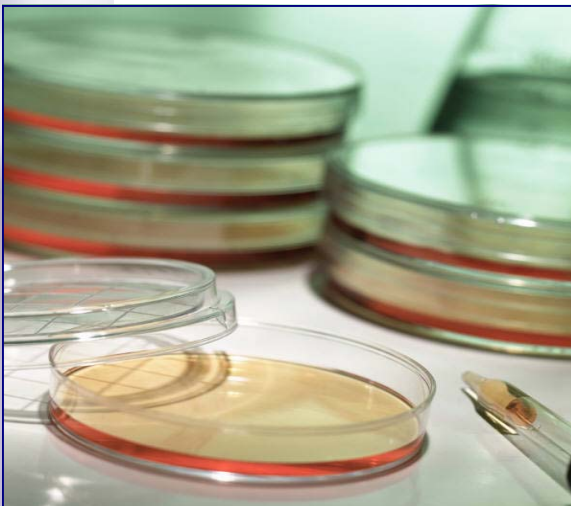
ASTM C1338 determines the ability of new insulation materials and their facings to support fungal growth.
