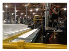
Polystyrene resin is expanded into foam from a pentane expanding agent and molded into profiles that are adhered to the vinyl siding. The insulated vinyl siding is then packaged and ready for distribution.
